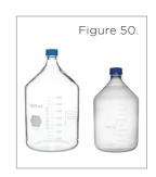
These solvent bottles are made from Type-33 borosilicate glass and have white enamel graduations and write-on patches. Due to their superior chemical stability, these bottles are useful for storage and delivery of reagents and both aqueous and/or organic solvents. Bottles with volumes of 100mL to 10L are supplied.
